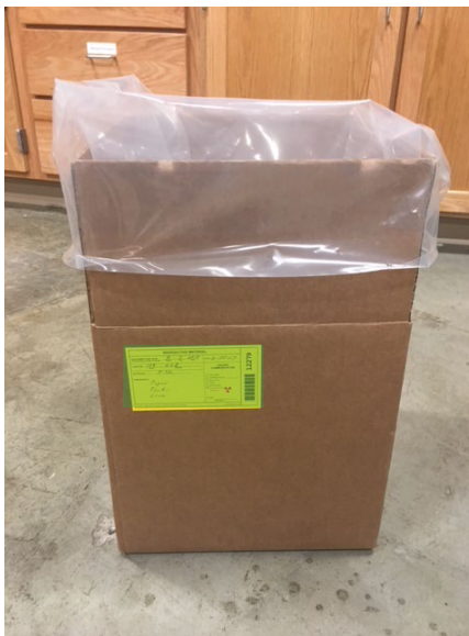
Figure 4. Example of liner appropriately placed inside cardboard box and labeled with HWL-R, ready for radioactive solid waste use.
