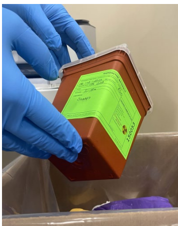
Figure 8. Once full, sharps containers can be placed directly into solid waste cardboard boxes with plastic liners as long as a biohazard is not also present.
