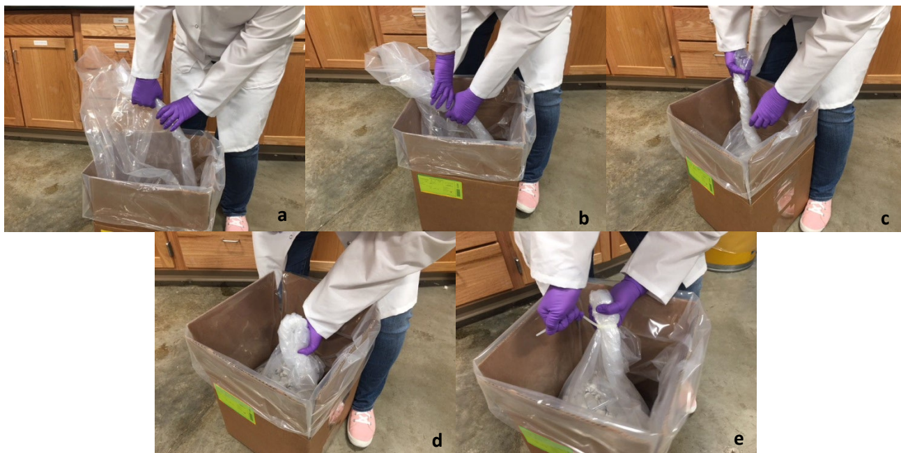
Figure 5a-e. How to properly and safety close and secure the plastic liner in a solid waste cardboard box container.
