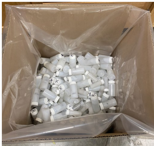
Figure 10. Close caps in LSC vials to prevent leakage. Separate LSC vials into their own solid waste cardboard box containers.
