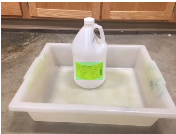
Figure 2. Liquid waste container stored appropriately in secondary containment.
